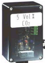
A detector with an infrared sensor for CO<sub>2</sub> measurings.
