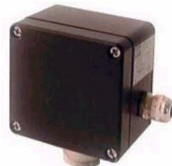
This gas detector is based on a zirconium cell, which has a longer operating life compared to common electrochemical cells – up to 5 years. This detector is more resistive to CO<sub>2</sub> than common electrochemical cells. Its measuring ranges are remarkable as well, not only the usual atmospheric range 0 – 25%, but also the measuring of the residual amount of oxygen 0 – 0,1%, or measuring in the range 0 – 96%.
